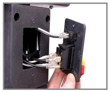
Figure 33. Power and light switch wiring.
